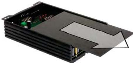
3. Release the indicated screws in order to remove the digital board.
