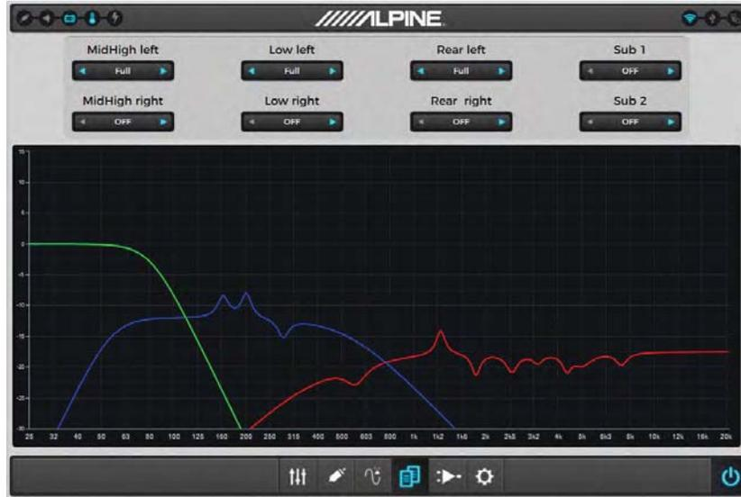
This screen visualizes the response curve(s) of the selected user adjustments of crossover, EQ, TCR and level for each output channel. The parameters and channels to be reflected in the visualization can be selected in the upper screen area by toggling the selection boxes.
