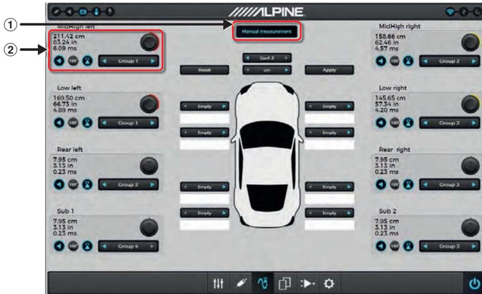
The time correction allows individual adjustments for each speaker output to align the different distances of each speaker relative to the listener's position inside the cabin. Adjustments can be done for level, delay and phase (0°/180°)
