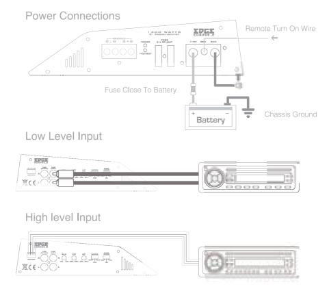
**NOTE**: When using high level input it is not necessary to connect the remote turn on whe. Do not connect both high level and low level input at the same time.
