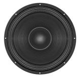
This next evolution subwoofer uses a new, longer, four layer aluminum voice coil. The result is less heat, more energy in the gap, higher sensitivity, higher power handling, lower distortion and better overall performance. The 18DS100 features a 34mm long, 4 inch diameter (100mm) Copper Clad Aluminum Wire voice coil. With a 1500watt AES power rating, 97.5 dB sensitivity, and over 14.0mm of Xvar, this high energy subwoofer is a significant step forward from similar models in the B&C range.
